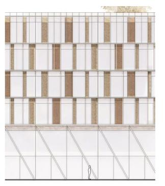
The upper part of the façade consists of an alternating rhythm of windows and solid metal elements. Thin metal fins shade the facade and give it depth.
